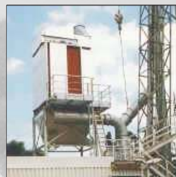
dedusting of a lime toploader kiln
