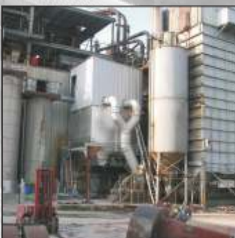
dedusting of rotary kiln during manufacture of perlite (stainless steel)
