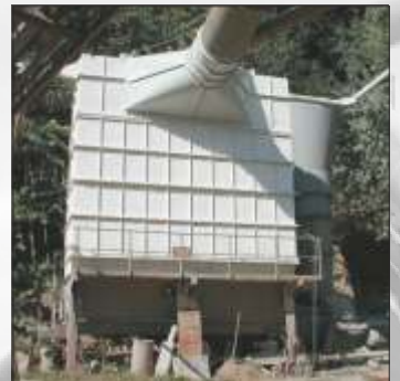
modern pressurised-air cleaned FB oval hose filter
