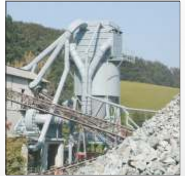
dedusting crushing and screening plant 130.000 Bm 3 /h
