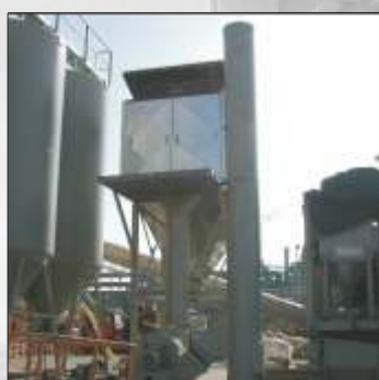
dedusting of a dry drum during manufacture of blasting material
